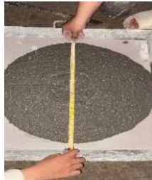
Gambar 3. Proses Uji Slump Flow
